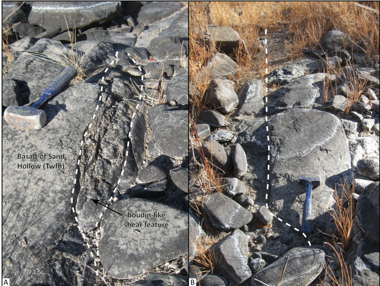
Figure 7-2. Fault breccia in Columbia River Basalt in the Dufur area. (a) A boudin-like zone of brecciated basalt intervening along the boundaries of columnar joint sets in the upper part of the Basalt of Sand Hollow (Twfh) along lower Pine Creek near Dufur (45.440301, -121.131046). (b) Planar zone of brecciated basalt cutting across columnar joint sets in the upper part of the Basalt of Sand Hollow (Twfh) in lower Pine Creek near Dufur (45.440629, -121.130771). Hammer for scale in both photographs is 25 cm (9.8 in) tall. Photo credits: J.D. McClaughry, 2016.
